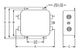
Typical dimensions: Terminals: .250 [*6.35*] (5) Slot: .07 x .16 [*1.8 x 4.1*]
