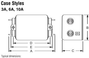
Terminals: .250 [*6.35*] (5) Slot: .07 x .16 [*1.8 x 4.1*] Holes: .07 [*1.8*] Dia.(4) Mounting holes: .188 [*4.78*] Dia. (2)
